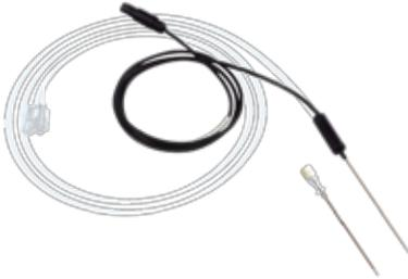
The disposable probe is 18 gauge with a 5.5 mm active tip. Probe includes a 4-foot connecting cable and tubing extension to reach out of the sterile field. These are connected to the generator and peristaltic pump unit for RF energy delivery and internal cooling.
